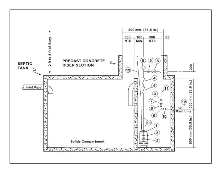
2. The effluent pump, to be supplied by the property owner for installation in the septic tank as shown in the diagram above, shall meet the standards and specifications of the "Hydromatic" submersible effluent pumps (SPD50H and SKHD 150) installed during the original installation of the sanitary sewage collection system. The effluent pump shall not have less than ½ horsepower or more than 1½ horsepower and they must be approved by the building inspector of the Regional District.
