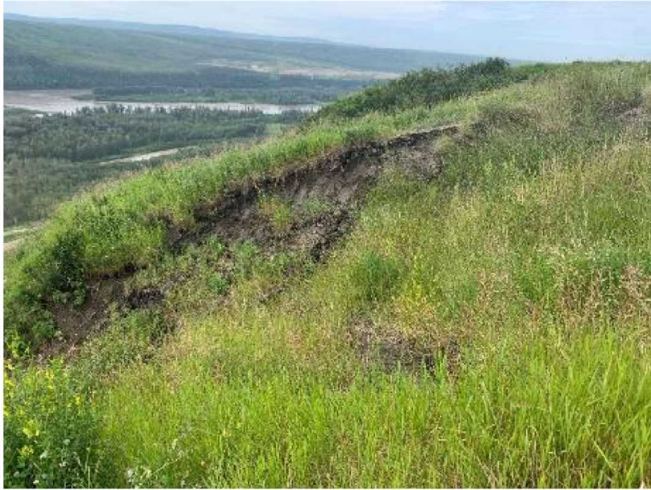
Photo 27: Surficial slope instabilities adjacent to viewpoint. July 7, 2020
