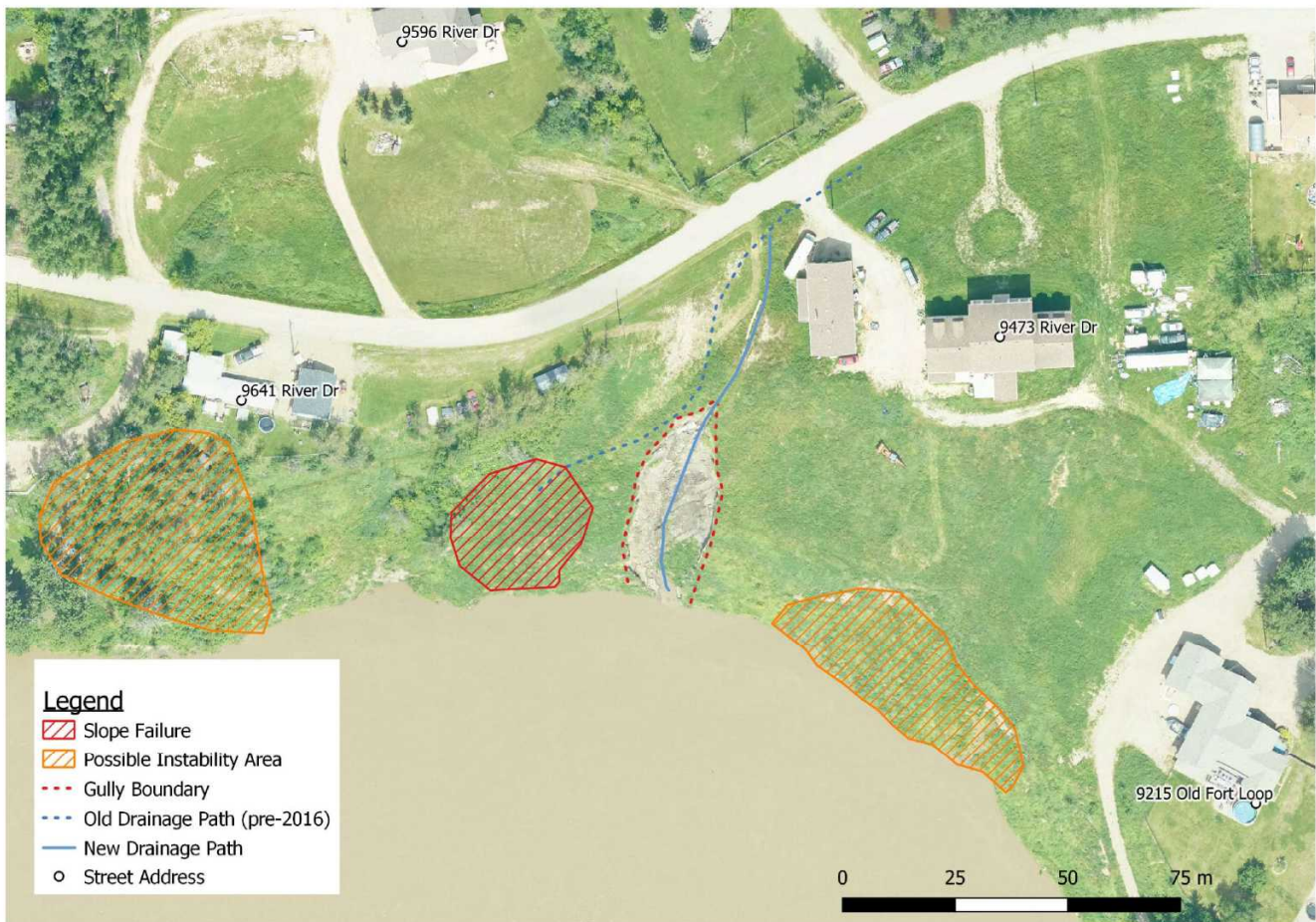
Figure 6: Gully forming south of River Drive on Peace River slope
