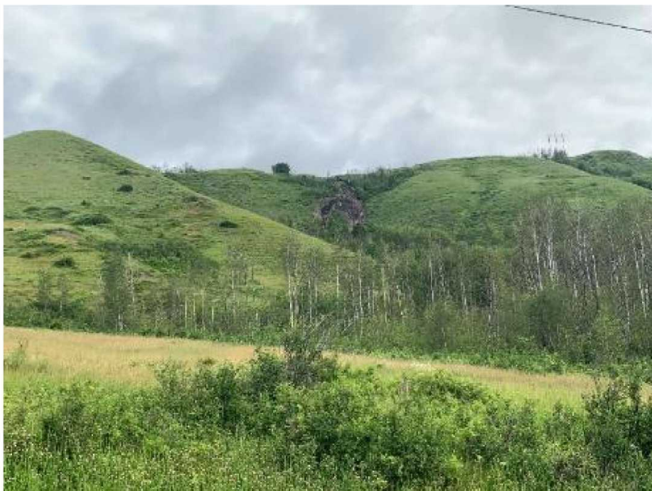
Photo 31: Surficial flow failure on south facing slopes west of 2018/2020 landslide . July 8, 2020
