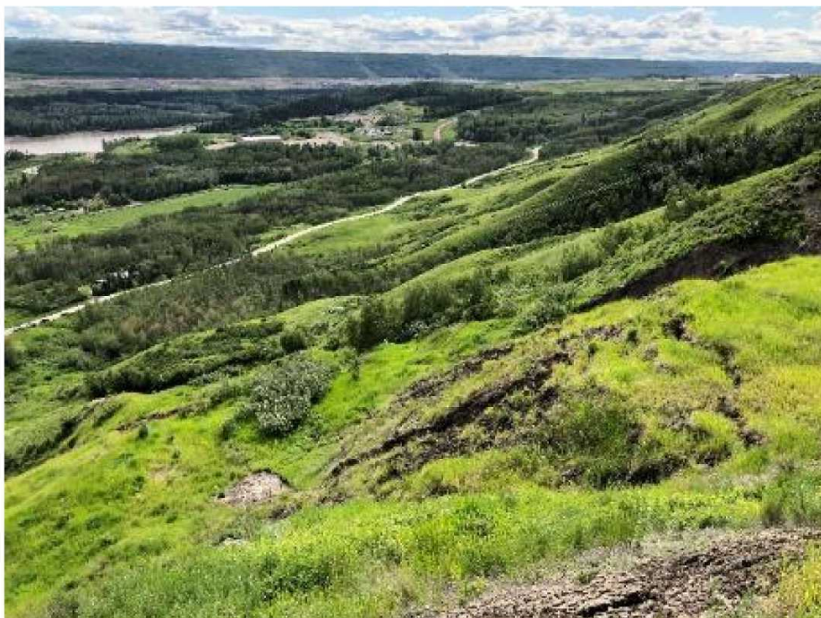
Photo 7: Slope relaxation and deformation on the steep slopes near the south end of the look-out. June 20, 2020
